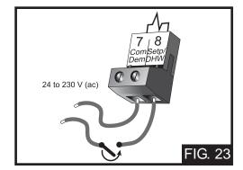
The boiler target temperature during a set point demand is increased to at least the Set Point setting. This temperature is maintained as long as the control has a set point demand.
